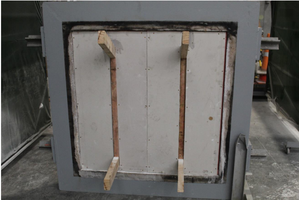
Fig.4 – Exposed face prior to fire stopping application
